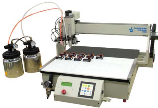
Dual Head Ink / Paint Applicator 24" x 15" Work Area Pallet system streamlines production by allowing operator to load/unload a 2 nd pallet during machine cycle. With Center-Shift software controlled valve shuttle.
