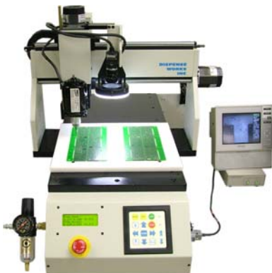
PC Board Rework and R&D Benchtop machining with control and features to satisfy most applications.
