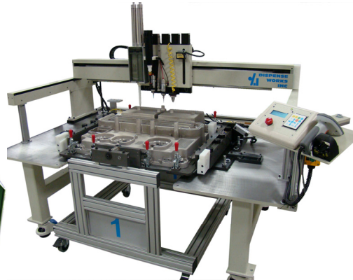
RG 7236 w/ 5 Heads and Cart Docking Dispensing 2 part epoxy, RTV, Laser inspection & serializing ID marking.
