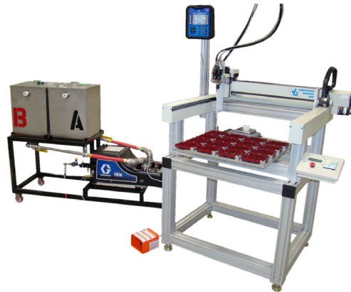
RG 2424 with 2 Part Epoxy System Gantry system with changeover pallets for step & repeat production. Also accommodates conveyors.
