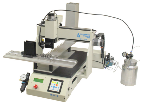
Custom Magazine Tooling and Assembly Glass slides shuttled and plastic discs are assembled with UV adhesive system.
