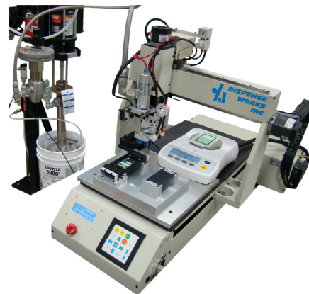
RP 1215 RTV Valve, and Pick & Place With 5gallon pail pump, laser sensor and scale for shot size verification.
