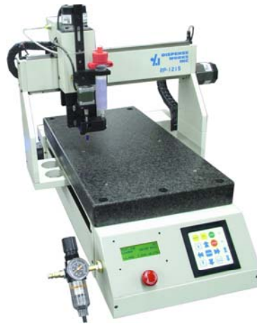
Ultra Precise 2" thick Granite Base System Unique programmable brushless auger valve directly controlled by system vector speed. A perfect flat and stable work surface.
