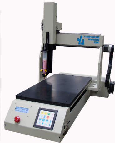
RP 1215 with Universal Syringe Mount Accommodates 5 – 10 – 30 – 55cc industry standard syringes. Removable on dovetail.
