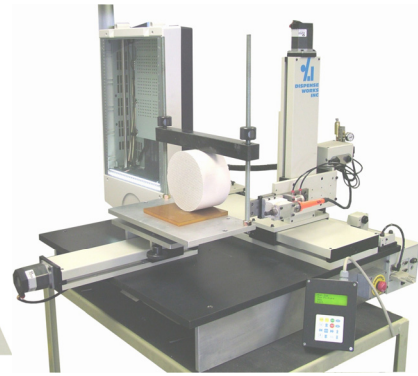
Custom Configuration Scans honeycomb part with scanner & pierces selected cells with a tool.
