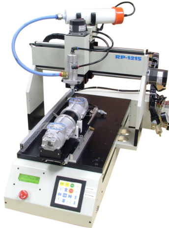
RTV Applicator with 2 stop Indexer Piggy back canister accommodates any standard caulk tube.
