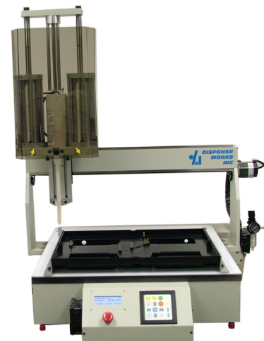
RP-2415 with 380ml 2 part cartridge Adhesive application with standard cartridge holder featuring quick change-over system.
